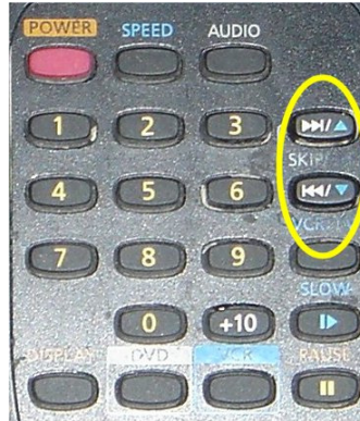
Fig. 7 Example of a remote control device using a two-button configuration for four directions. Notice that the mapping of direction to the button configurations is congruent with our results.
